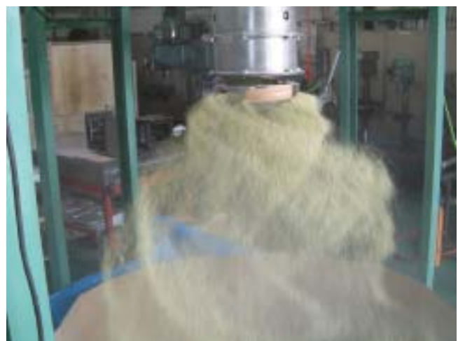
Catalyst loading demonstration using the catalyst loading machine
