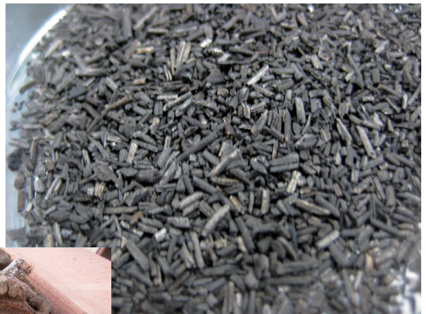
Activated carbons made from the trunks of date trees
