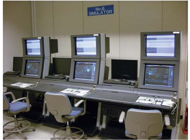
Old training simulator (upgraded in 2001; Yamatake Advanced-PS R530 DCS)
