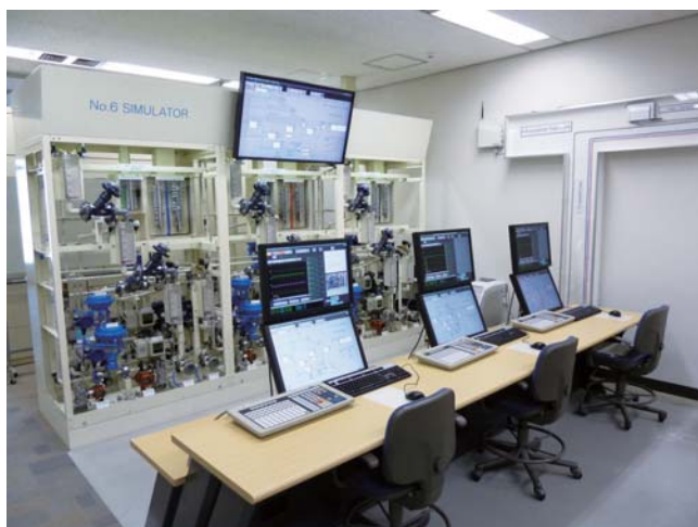
New training simulator (upgraded in 2011; Yamatake Harmonas-DEO R400 DCS)
